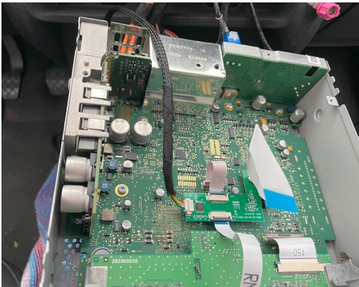
***Step 7. Connect the video cables of the interface (plugs)***
