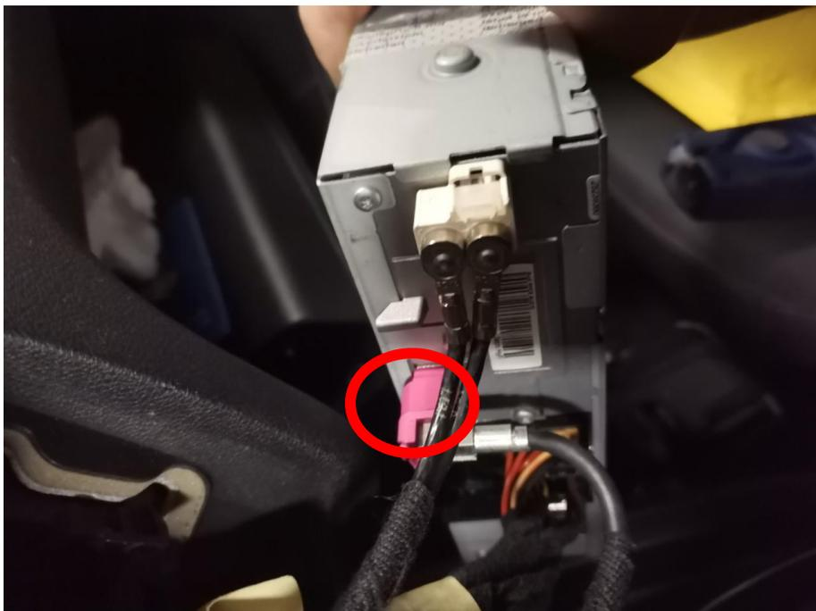
Press the pink video connector at the bottom into the latch. Pry very gently with a small flat object between the seam if the plug is very tight. This is where
